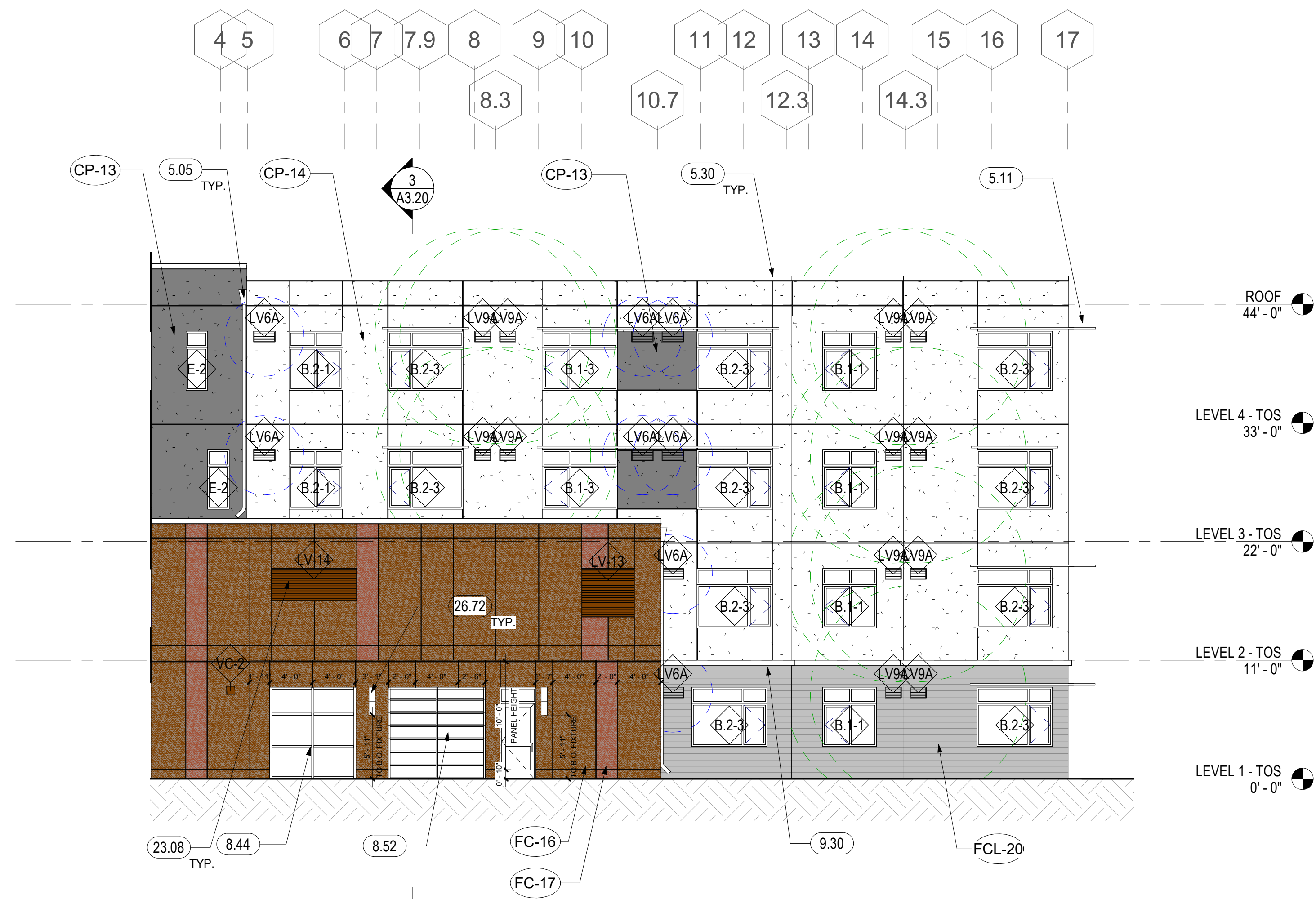
2 PSH 2 - WEST ELEVATION 1/8" = 1'-0"
